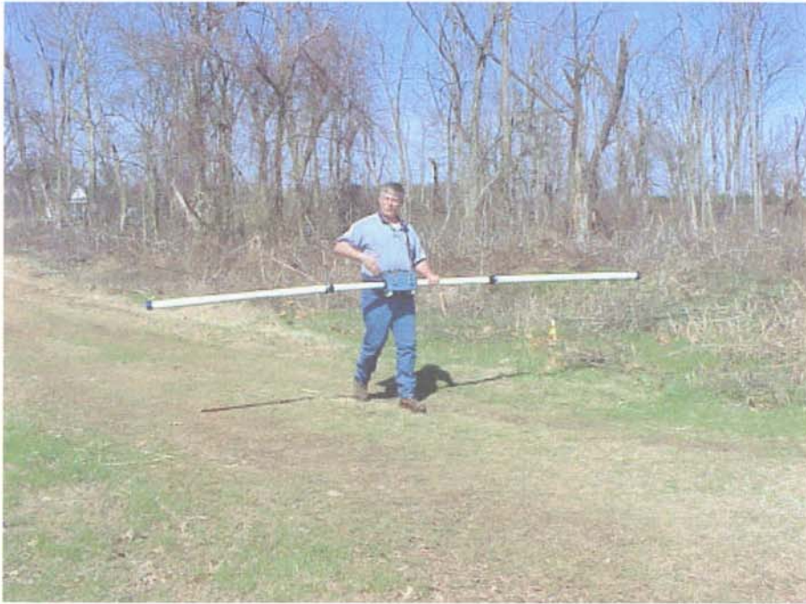
Figure 7. Conductivity survey by geologist at Stop 6. Upper photograph is view looking southeast, near edge of old abandoned course. Lower photograph is view looking north at Bakers Bayou in background. At this location, there is no well-defined channel
