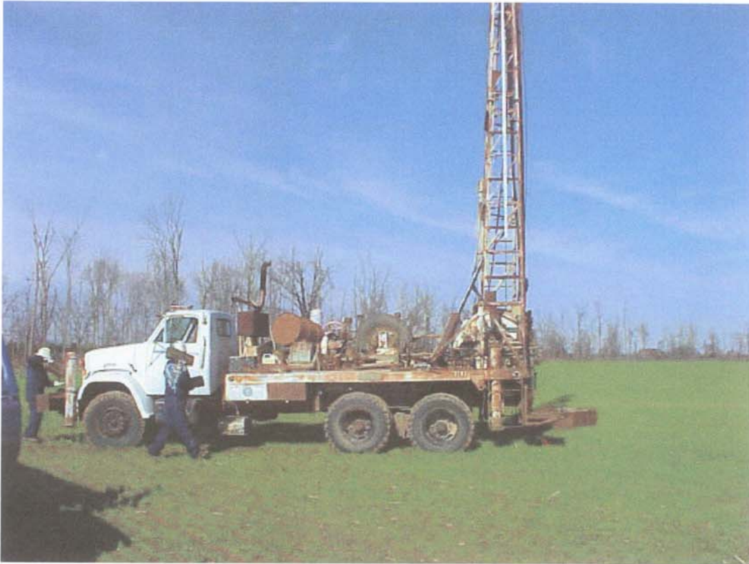
Figure 6. Drilling equipment used to sample at Bakers Bayou, Stop 6. Drill rig is set up within the old channel of the abandoned Arkansas River Course. Tree line in background corresponds to the present day bayou
